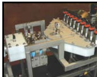
Metering Pump, Manifold, and Valves
